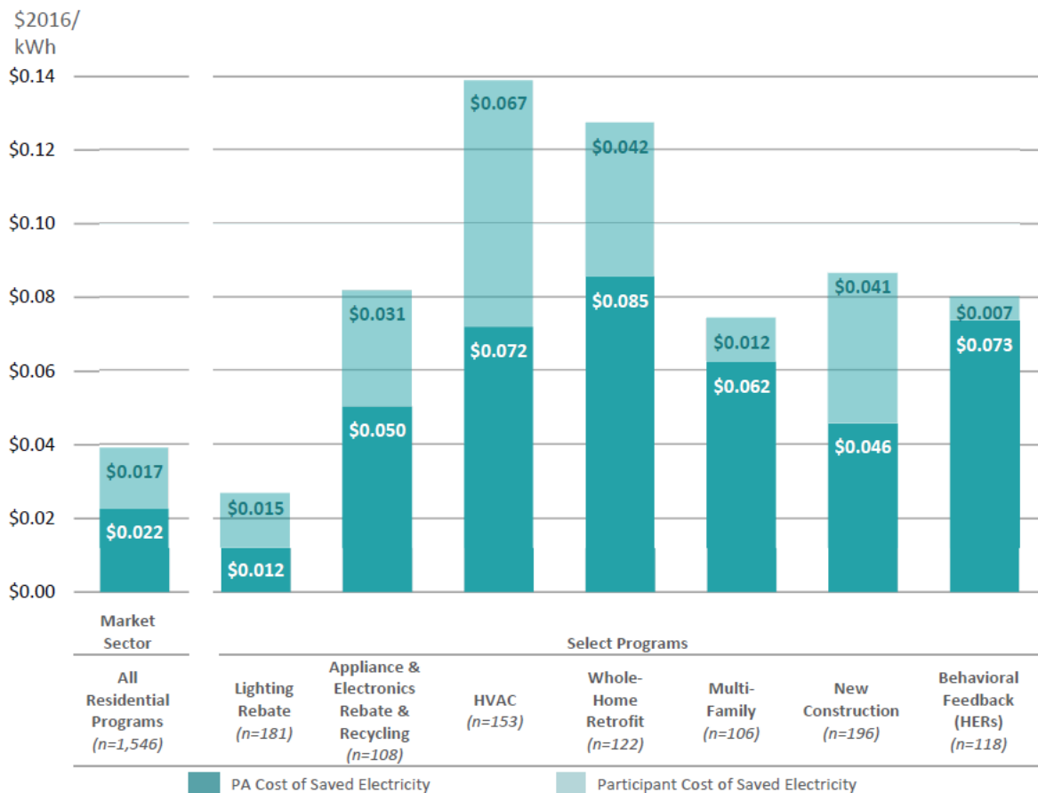
Figure 18: Average total costs (program administrator (PA) + participant costs) of saved electricity by residential program type. Source: LBNL: The Cost of Saving Electricity Through Energy Efficiency Programs Funded by Utility Customers: 2009–2015. June 2018. http://eta-publications.lbl.gov/sites/default/files/cose_final_report_20180619_1.pdf
