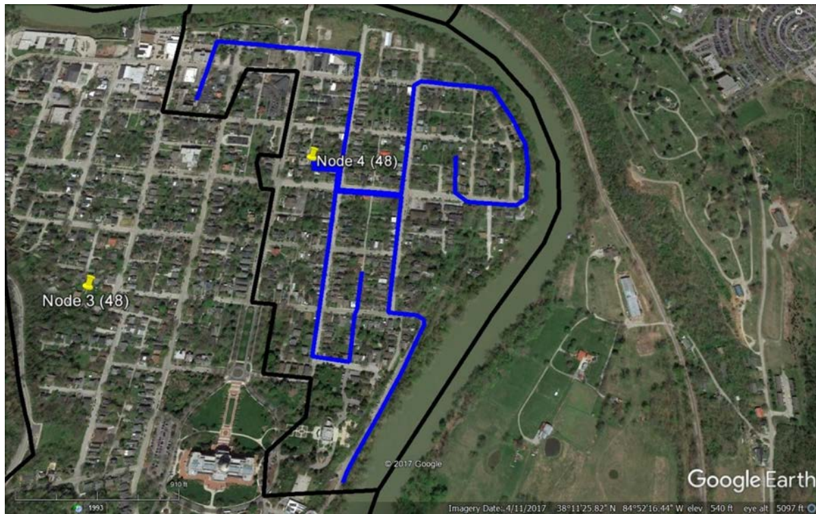
Figure 17-3: Typical FTTH Urban Design
