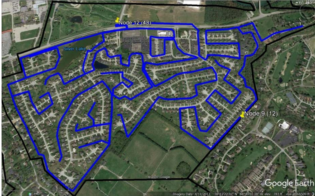
Figure 17-1: Typical FTTH Dense Suburban Design
